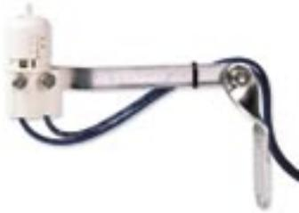
The standard Mini-Klik model, for use in most applications. Constructed of high impact thermoplastic and aluminum. Simple klik-stop settings accurately measure rainfall in quantities of 1/8" to 1". Reset rate is adjustable. Model: MINI-CLIK
